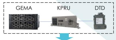
Key Processor (KPRU): Hardware with crypto generation capabilities. Fully-developed by TECNOBIT, it implements the cryptography to protect the input and output of cypher keys.
